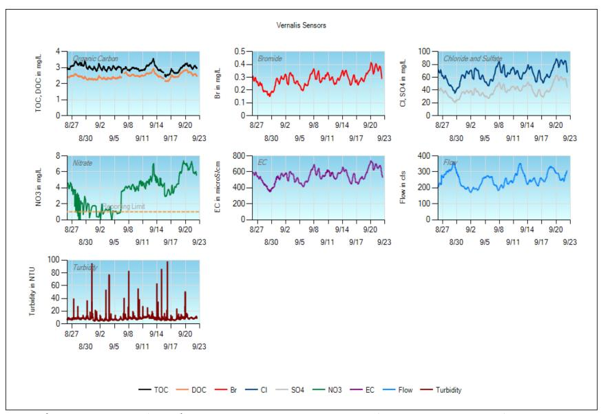
**Events: 9/6** = Replaced 50 micron filter. **9/15** = QC event, replaced 50, 1, and 0.45 micron filters. Added 100 micron pre-filter. Cleaned the pump intake. **9/21** = Replaced 100 micron filter. Made new check standard for the Dionex.
