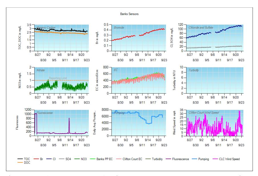
**9/2** – Removed 100 um filter and cleaned 50 um pleated filter. **9/7** – Installed new columns on the anion analyzer, initiated calibration. **9/8** – Cleaned 50 um filter. **9/14** – Cleaned 50 um filter and rinsed 0.45 um filter. **9/21** – Changed 1 um filter and cleaned 50 um pleated filter.
