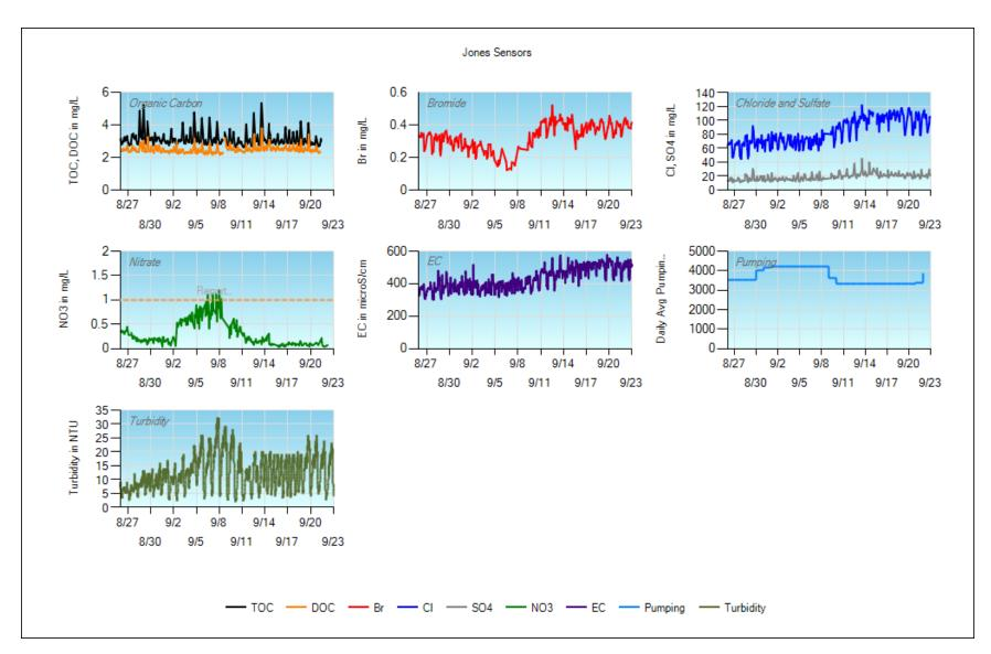
**9/2** – Filter change **9/8** – Filter change. Added a double in-line guard column to the Dionex. By doing this, bromide peaks have shifted away from the contamination peak. Bromide peaks appear to be more symmetrical and check standard values more accurate. **9/14** – Filter change **9/21** – Filter change. Flow magnet stuck causing erroneous organic carbon data. Nitrate continues to report below the reporting limit.
