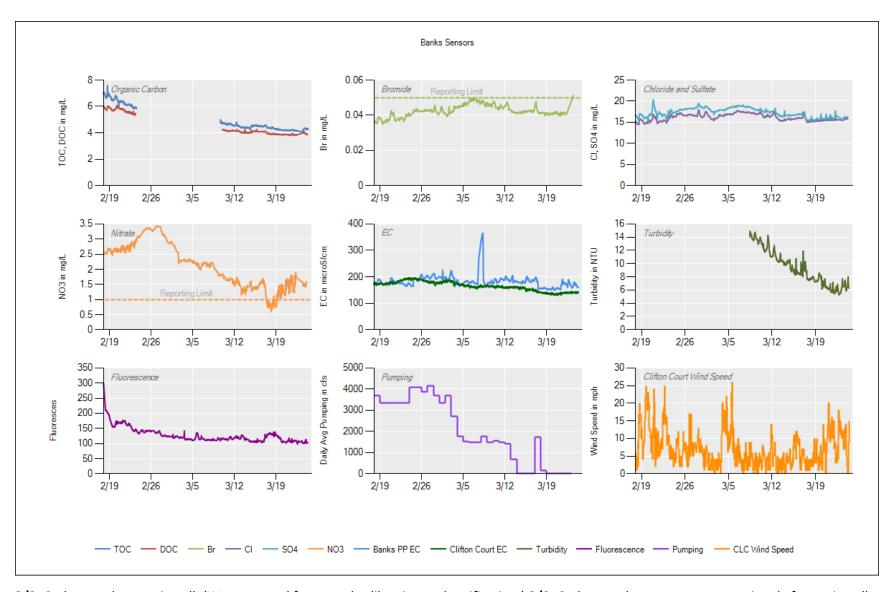
**3/2:** Carbon analyzer re-install. (Was removed for annual calibration and verification.) **3/9:** Carbon analyzer was non-operational after re-install, troubleshot issue, re-started. **3/23:** Computer was down, possible power outage; re-started. Changed the 100 and 0.45 um filters. Rinsed the 50 um filter.
