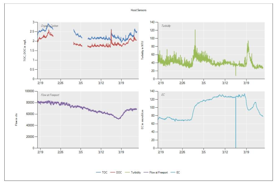
**3/2:** Carbon analyzer re-install. **3/6:** Power outage **3/15:** Analyzed all QC samples, changed all filters. (50, 1 and 0.45 um) **3/23:** Rinsed the 50 um filter.
