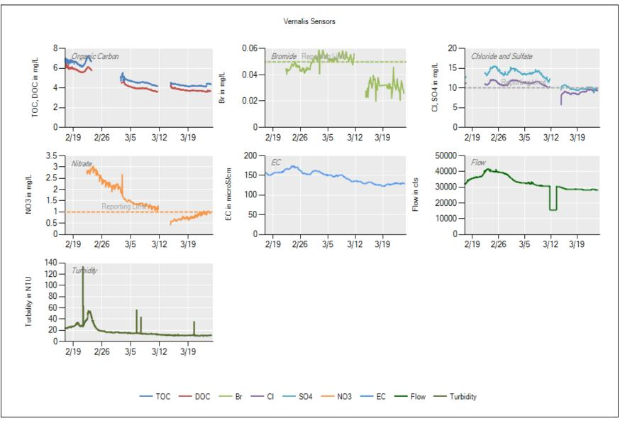
Events: Dionex 2/17 - 2/22 = Program/start sequence problem. 3/11 - 3/14 = Air bubbles entered pump system through DI reservoir. Sievers 2/23 - 3/3 = Removed for annual calibration and verification. 3/11 - 3/14 = Data logging program glitch. Data is available for the time period.
