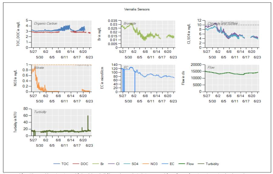
**Events:** 6/1 = Filter and housing rinse. 6/13 = QC and all filters changed. Debris removed from front of station. Pump intake cleaned. IOS/sampling manifold for carbon analyzer cleaned. **Note:** Still having problem with valves for sampling manifold on the Sievers carbon analyzer. Site visit planned for afternoon of Friday 6/23 (after this graphical update was produced).
