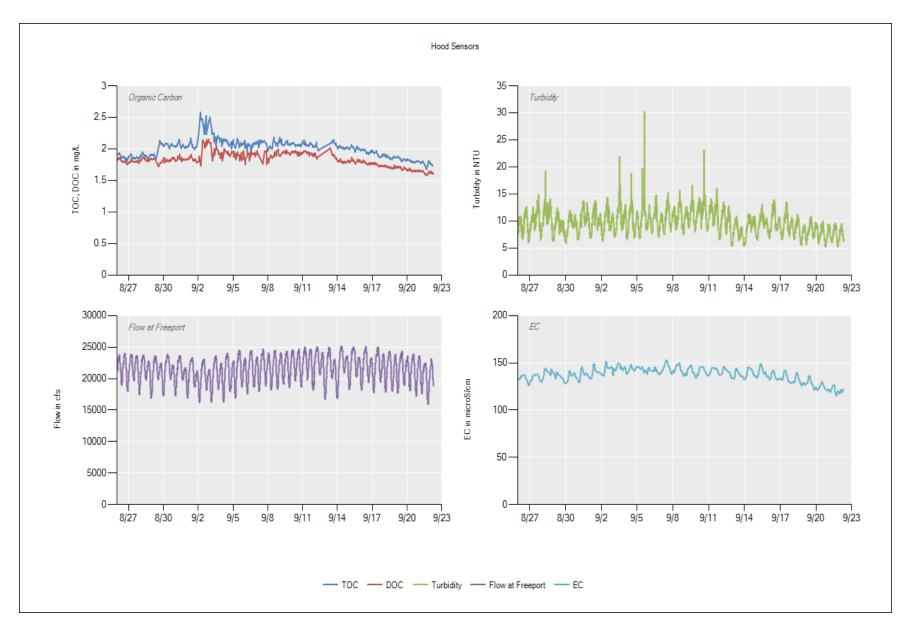
8/29 – Replaced the 50 and 1 um filters. 9/12 – Consumable component depleted.
