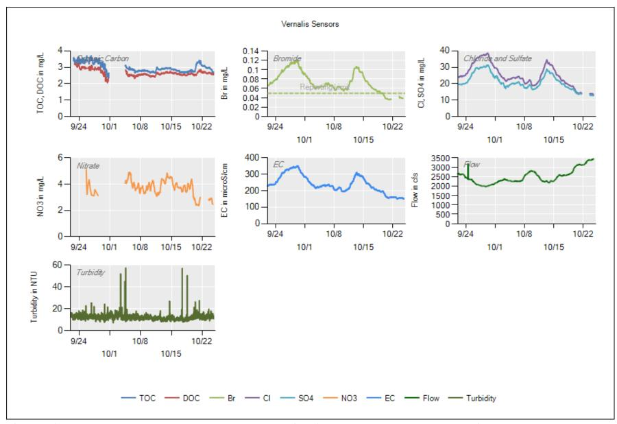
9/23 = TOC/DOC results overlap from a leaking valve (data edited). 10/1-10/4 = Clog in the Sievers sample inlet. 10/22 = Dionex software glitch.
