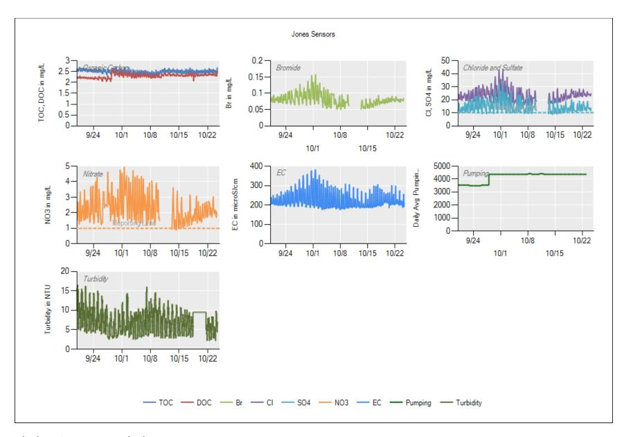
9/28/17 – filter change. 10/10/17 – The Dionex eluent generator was replaced and the Dionex was recalibrated. Filter change.
