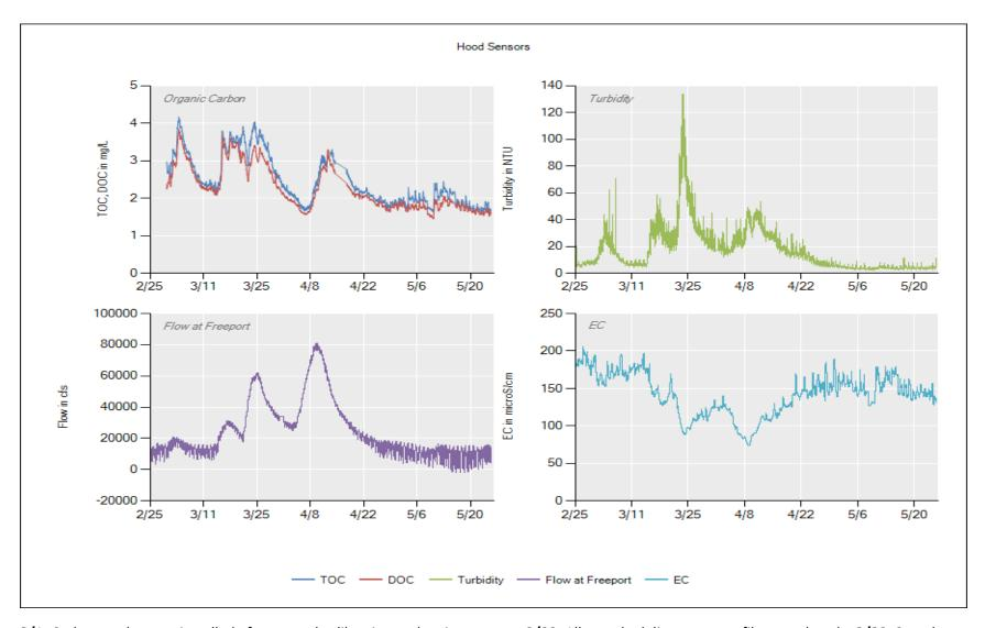
**3/1:** Carbon analyzer re-installed after annual calibration and maintenance – **3/20:** All sample delivery system filters replaced – **3/30:** Sample pump float partially submerged, lifted out of water and reset – **4/9:** Pump partially submerged again, pulled up and reset – **4/17:** Replaced all sample delivery system filters – **5/3:** Replaced 50 um filter – **5/15:** Cleaned 50 um filter, replaced the 1 and 0.45 um filters
