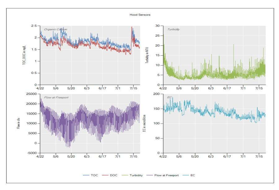
5/3 to 7/17: Normal station and sample delivery system maintenance and QC over the time period. Replaced analyzer consumables on 7/17.
