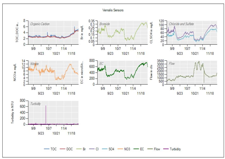
New Events: Filter Changes: 10/30, 11/15, 11/28. New pump seals for the Dionex on 11/28. Goodwin releases ramp up beginning 10/16 to 11/3.
