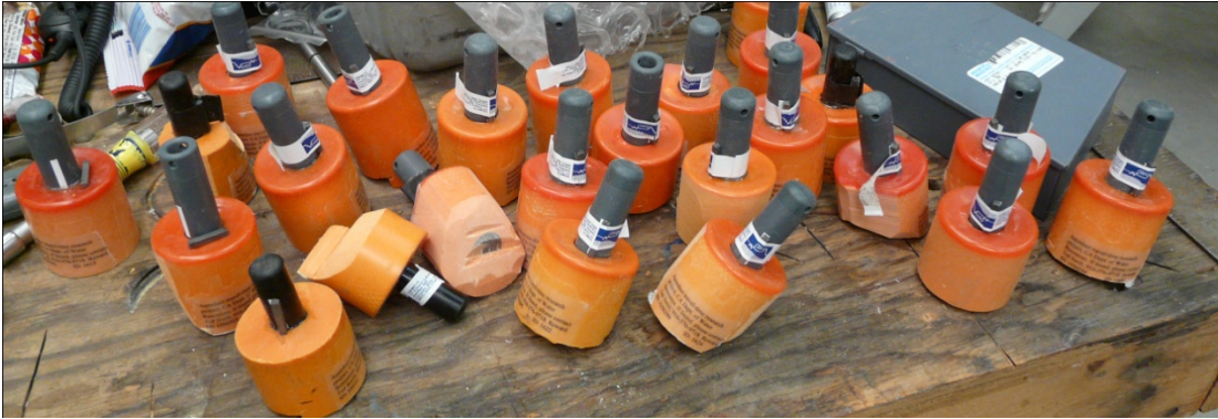
Photo 1: Neutrally buoyant drifters being manufactured at the MWQI Field Support shop. The orange floats are approximately 2 inches (5 cm) long. The cylindrical black acoustic tags are embedded in the bottom ends of the orange drifters.
