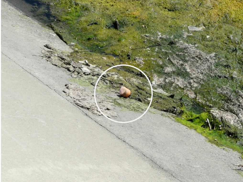
Photo 2: A drifter found entangled in a mass of algae on the side of the aqueduct. This drifter was recovered thanks to the sharp eyes of one of the investigators. The drifter is approximately 2 inches (5 cm) long. The cylindrical black acoustic tag is embedded in the bottom end of the drifter (not visible).
