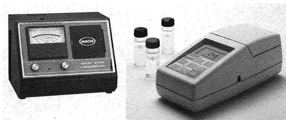
PHOTO 11: Hach Nephelometers: (left): 2100A Model (right): 2100P Model (both from Hach Co.).
