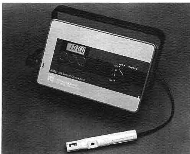
PHOTO 7: Dissolved Oxygen Meter (from YSI Inc.).
