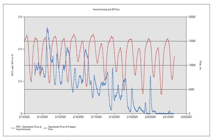
12/18: Reinstalled the ammonia analyzer – 2/13: Started the ammonia analyzer, flushed the system, after some adjustments and troubleshooting was able to calibrate, analyzed a single check standard, 1.0 ppm which reported 1.05 ppm, started analyzing Sacramento River water
