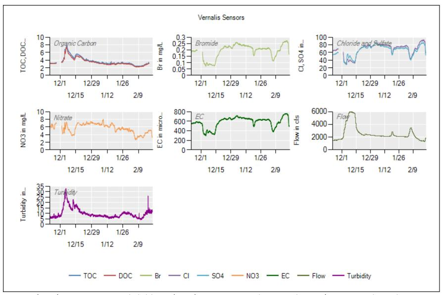
**Events:** 11/27-12/2 = Power outage over the holiday. 12/1 - 12/15 = precipitation and reservoir releases. 2/18 = organic carbon analyzer removed for annual service/calibration.
