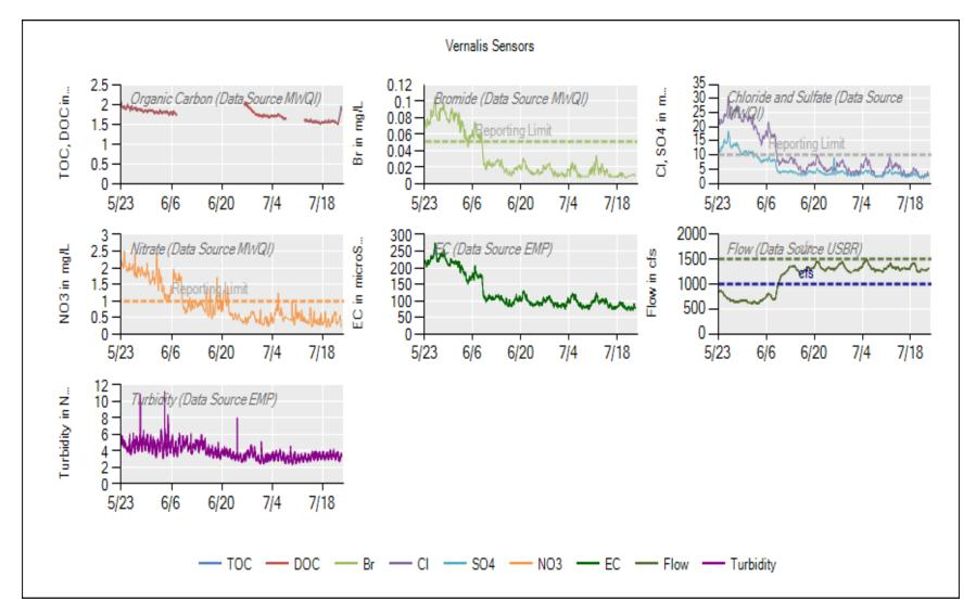
6/29: Fixed an issue with carbon analyzer sample flow -7/1: Had to reconnect stream communication wires on the carbon analyzer and turn the streams setting back on, switched the motherboard connection wires, changed the clock to PST, it was set to DST, removed a pressure increasing line on the anion analyzer to decrease the pressure -7/9: Computer was off so it was restarted -7/22: Replaced all sample delivery system filters
